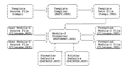
Figure 1-1 Model for M2FORMAT Software
